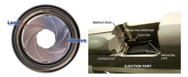
When bullets are propelled forward through a barrel they may take on the inverse of the lands and grooves (respectively peaks and valleys) of its rifling as well as the imperfections/ scratches (striations or striae) within those lands and grooves; cartridge cases may in turn be marked by the surfaces they impact, such as a gun's breech face and firing pin. Id. at 7-8.
